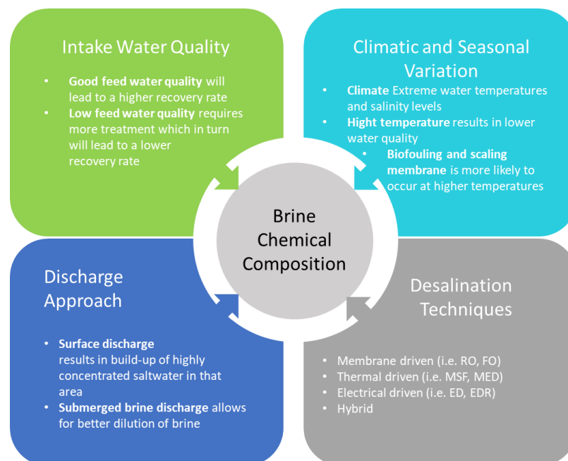
Figure 2: Influences on the physiochemical characteristics of discharged brine, recreated from Omerspahic et al., 2022 [10]
